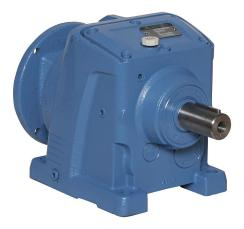
IronHorse heavy-duty helical gearbox, 30:1 ratio, 145TC-Face input, inline, 1.25in diameter output shaft, nominal 2hp at 1.0 SF, 2080 lb-in mechanical output torque, Type-47 frame, cast iron housing, foot mount.
