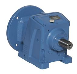
IronHorse heavy-duty helical gearbox, 20:1 ratio, 182TC-Face input, inline, 1.25in diameter output shaft, nominal 3hp at 1.0 SF, 1860 lb-in mechanical output torque, Type-47 frame, cast iron housing, foot mount.
