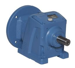
IronHorse heavy-duty helical gearbox, 15:1 ratio, 182/4TC-Face input, inline, 1.25in diameter output shaft, nominal 3hp at 1.0 SF, 1520 lb-in mechanical output torque, Type-47 frame, cast iron housing, foot mount.
