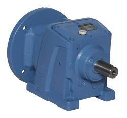
IronHorse heavy-duty helical gearbox, 10:1 ratio, 182/4TC-Face input, inline, 1.25in diameter output shaft, nominal 3hp at 1.0 SF, 1140 lb-in mechanical output torque, Type-47 frame, cast iron housing, foot mount.
