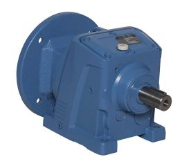
IronHorse heavy-duty helical gearbox, 5:1 ratio, 182/4TC-Face input, inline, 1.25in diameter output shaft, nominal 3hp at 1.0 SF, 490 lb-in mechanical output torque, Type-47 frame, cast iron housing, foot mount.
