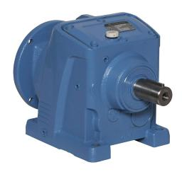
IronHorse heavy-duty helical gearbox, 5:1 ratio, 145TC-Face input, inline, 1.25in diameter output shaft, nominal 2hp at 1.0 SF, 330 lb-in mechanical output torque, Type-47 frame, cast iron housing, foot mount.
