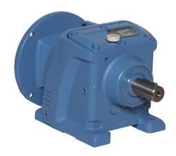
IronHorse heavy-duty helical gearbox, 60:1 ratio, 56C-Face input, inline, 1in diameter output shaft, nominal 0.82hp at 1.0 SF, 1770 lb-in mechanical output torque, Type-37 frame, cast iron housing, foot mount.
