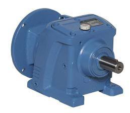
IronHorse heavy-duty helical gearbox, 30:1 ratio, 56C-Face input, inline, 1in diameter output shaft, nominal 1hp at 1.0 SF, 1010 lb-in mechanical output torque, Type-37 frame, cast iron housing, foot mount.
