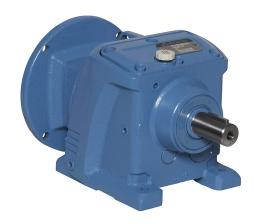
IronHorse heavy-duty helical gearbox, 20:1 ratio, 145TC-Face input, inline, 1in diameter output shaft, nominal 2hp at 1.0 SF, 1350 lb-in mechanical output torque, Type-37 frame, cast iron housing, foot mount.
