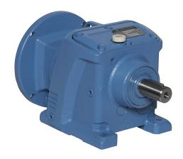
IronHorse heavy-duty helical gearbox, 15:1 ratio, 145TC-Face input, inline, 1in diameter output shaft, nominal 2hp at 1.0 SF, 950 lb-in mechanical output torque, Type-37 frame, cast iron housing, foot mount.
