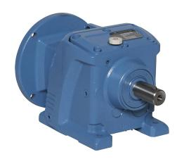
IronHorse heavy-duty helical gearbox, 10:1 ratio, 145TC-Face input, inline, 1in diameter output shaft, nominal 2hp at 1.0 SF, 670 lb-in mechanical output torque, Type-37 frame, cast iron housing, foot mount.
