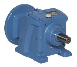
IronHorse heavy-duty helical gearbox, 5:1 ratio, 145TC-Face input, inline, 1in diameter output shaft, nominal 2hp at 1.0 SF, 330 lb-in mechanical output torque, Type-37 frame, cast iron housing, foot mount.
