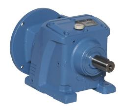
IronHorse heavy-duty helical gearbox, 5:1 ratio, 56C-Face input, inline, 1in diameter output shaft, nominal 1hp at 1.0 SF, 160 lb-in mechanical output torque, Type-37 frame, cast iron housing, foot mount.
