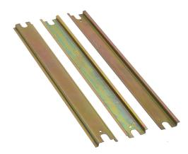
Wiegmann DIN rail, 35mm, 7.5mm height, 14in length, plated steel. Package of 3. For use with 16in high or wide N412 Ultimate series enclosures.
