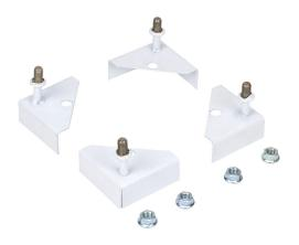
Wiegmann enclosure panel conversion kit, white, polyester powder finish, allows standard NP series sub panels to mount in Ultimate series enclosures up to 30 x 30in (HxW) nominal size, includes (4) brackets and mounting hardware.
