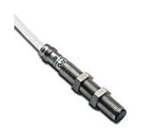
AutomationDirect photoelectric sensor, tubular, threaded, stainless steel housing, through-beam receiver, 1m sensing distance, 10-30 VDC operating voltage, light-on, PNP, 3-wire, pigtail.
