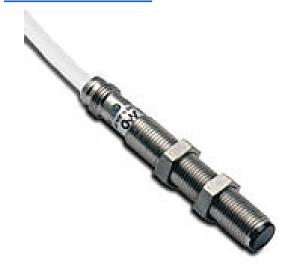
AutomationDirect photoelectric sensor, tubular, threaded, stainless steel housing, through-beam receiver, 1m sensing distance, 10-30 VDC operating voltage, light-on, NPN, 3-wire, pigtail.
