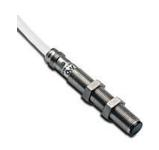
AutomationDirect photoelectric sensor, tubular, threaded, stainless steel housing, through-beam receiver, 1m sensing distance, 10-30 VDC operating voltage, light-on, NPN, 3-wire, pigtail.
