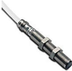
AutomationDirect photoelectric sensor, tubular, threaded, stainless steel housing, through-beam receiver, 1m sensing distance, 10-30 VDC operating voltage, light-on, NPN, 3-wire, pigtail.
