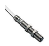
AutomationDirect photoelectric sensor, tubular, threaded, stainless steel housing, through-beam receiver, 1m sensing distance, 10-30 VDC operating voltage, dark-on, PNP, 3-wire, pigtail.
