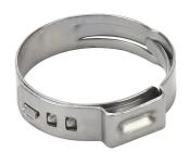
NITRA hose clamp, interlocking ear, 0.823-0.949in diameter, 304 stainless steel. Package of 10. For use with HBV series 5/8in hose.
