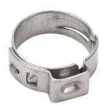
NITRA hose clamp, interlocking ear, 0.398-0.465in diameter, 304 stainless steel. Package of 10. For use with HBV series 1/4in hose.
