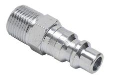
NITRA pneumatic quick disconnect fitting, coupling plug, steel body, (1) 3/8in male NPT to (1) 3/8in industrial interchange.
