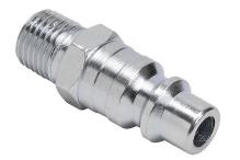
NITRA pneumatic quick disconnect fitting, coupling plug, steel body, (1) 1/4in male NPT to (1) 3/8in industrial interchange.
