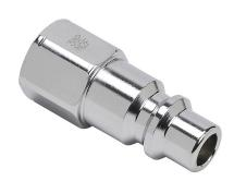
NITRA pneumatic quick disconnect fitting, coupling plug, chromeplated steel body, (1) 1/4in female NPT to (1) 3/8in industrial interchange.
