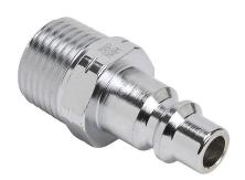
NITRA pneumatic quick disconnect fitting, coupling plug, chromeplated steel body, 3/8in industrial interchange to 1/2in male NPT.
