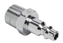
NITRA pneumatic quick disconnect fitting, coupling plug, chromeplated steel body, (1) 3/8in male NPT to (1) 1/4in industrial interchange.
