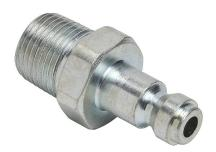
NITRA pneumatic quick disconnect fitting, coupling plug, steel body, (1) 3/8in male NPT to (1) 1/4in Truflate.
