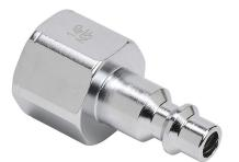
NITRA pneumatic quick disconnect fitting, coupling plug, chromeplated steel body, (1) 3/8in female NPT to (1) 1/4in industrial interchange.
