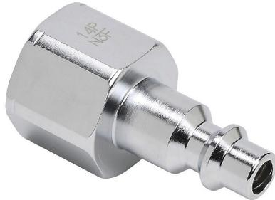
NITRA pneumatic quick disconnect fitting, coupling plug, chrome-plated steel body, (1) 3/8in female NPT to (1) 1/4in industrial interchange.
