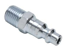
NITRA pneumatic quick disconnect fitting, coupling plug, steel body, (1) 1/4in male NPT to (1) 1/4in industrial interchange.
