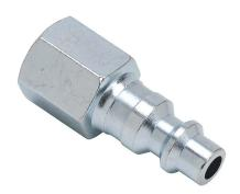
NITRA pneumatic quick disconnect fitting, coupling plug, steel body, (1) 1/4in female NPT to (1) 1/4in industrial interchange.
