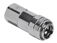
NITRA pneumatic quick disconnect fitting, automatic coupling, chrome-plated steel body, 3/8in industrial interchange to 3/8in female NPT.
