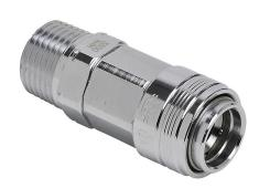
NITRA pneumatic quick disconnect fitting, automatic coupling, chrome-plated steel body, (1) 1/2in male NPT to (1) 3/8in industrial interchange.
