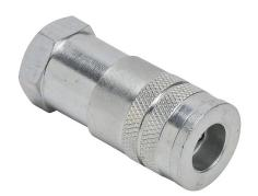
NITRA pneumatic quick disconnect fitting, coupling, steel body, (1) 3/8in female NPT to (1) 1/4in industrial interchange.
