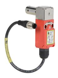
IDEM safety switch, hollow shaft hinge interlock, slow action, (2) N.C. safety output(s), plastic body, 316 stainless steel head, 16mm diameter x 30mm length shaft, (1) 4-pin M12 quick-disconnect.
