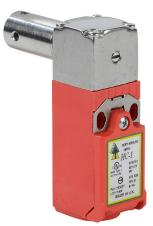
IDEM safety switch, hollow shaft hinge interlock, slow action, (2) N.C. safety output(s), plastic body, 316 stainless steel head, 16mm diameter x 30mm length shaft, (1) M16 cable entry.
