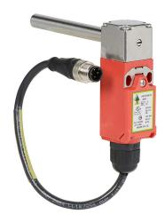
IDEM safety switch, solid shaft hinge interlock, slow action, (2) N.C. safety output(s), plastic body, 316 stainless steel head, 10mm diameter x 80mm length shaft, (1) 4-pin M12 quick-disconnect.
