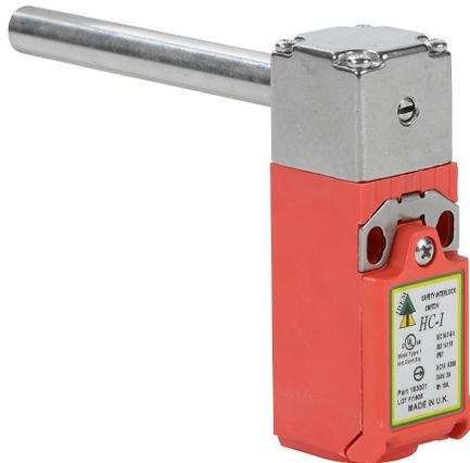
IDEM safety switch, solid shaft hinge interlock, slow action, (2) N.C. safety output(s), plastic body, 316 stainless steel head, 10mm diameter x 80mm length shaft, (1) M16 cable entry.
