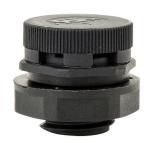
Bimed pressure relief vent plug, M12 x 1.5mm thread type, polyamide, black, 2,000 mL/min @ 70 mBar (1 psi), IP67 IP68, UL Type 4X, 12 and 13. Package of 2.
