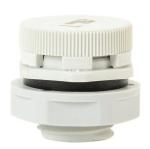
Bimed pressure relief vent plug, M12 x 1.5mm thread type, polyamide, light gray, 2,000 mL/min @ 70 mBar (1 psi), IP67 IP68, UL Type 4X, 12 and 13. Package of 2.
