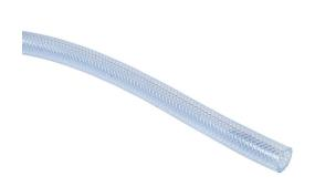
HydroMode potable water hose, polyester-reinforced PVC, clear blue, 5/8in inside diameter, 0.891in outside diameter, NSF/ANSI 61, 300ft reel.
