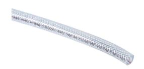
HydroMode potable water hose, polyester-reinforced PVC, clear blue, 5/16in (8mm) inside diameter, 0.531in outside diameter, NSF/ANSI 61, 300ft reel.
