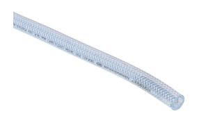
HydroMode potable water hose, polyester-reinforced PVC, clear blue, 3/8in inside diameter, 0.594in outside diameter, NSF/ANSI 61, 300ft reel.
