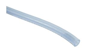
HydroMode potable water hose, polyester-reinforced PVC, clear blue, 3/4in inside diameter, 1.03in outside diameter, NSF/ANSI 61, 300ft reel.
