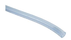
HydroMode potable water hose, polyester-reinforced PVC, clear blue, 3/4in inside diameter, 1.03in outside diameter, NSF/ANSI 61, 100ft package.
