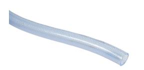
HydroMode potable water hose, polyester-reinforced PVC, clear blue, 1in inside diameter, 1.3in outside diameter, NSF/ANSI 61, 200ft reel.
