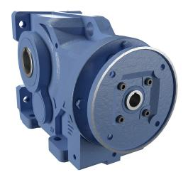
IronHorse heavy-duty helical bevel gearbox, 120:1 ratio, 182TC-Face input, hollow, 2.375in diameter output shaft, nominal 3hp at 2.08 SF, 23900 lb-in mechanical output torque, Type-87 frame, cast iron housing, vertical or horizontal mount.
