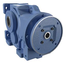
IronHorse heavy-duty helical bevel gearbox, 80:1 ratio, 182/4TC-Face input, hollow, 2.375in diameter output shaft, nominal 5hp at 1.74 SF, 23570 lb-in mechanical output torque, Type-87 frame, cast iron housing, vertical or horizontal mount.
