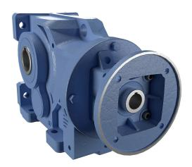
IronHorse heavy-duty helical bevel gearbox, 60:1 ratio, 213/5TC-Face input, hollow, 2.375in diameter output shaft, nominal 10hp at 1.11 SF, 22270 lb-in mechanical output torque, Type-87 frame, cast iron housing, vertical or horizontal mount.
