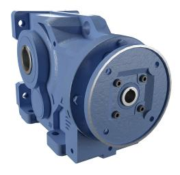
IronHorse heavy-duty helical bevel gearbox, 60:1 ratio, 182/4TC-Face input, hollow, 2.375in diameter output shaft, nominal 5hp at 2.22 SF, 22270 lb-in mechanical output torque, Type-87 frame, cast iron housing, vertical or horizontal mount.
