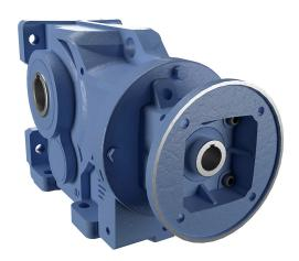
IronHorse heavy-duty helical bevel gearbox, 40:1 ratio, 213/5TC-Face input, hollow, 2.375in diameter output shaft, nominal 10hp at 1.48 SF, 20870 lb-in mechanical output torque, Type-87 frame, cast iron housing, vertical or horizontal mount.
