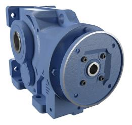
IronHorse heavy-duty helical bevel gearbox, 40:1 ratio, 182/4TC-Face input, hollow, 2.375in diameter output shaft, nominal 5hp at 2.95 SF, 20870 lb-in mechanical output torque, Type-87 frame, cast iron housing, vertical or horizontal mount.
